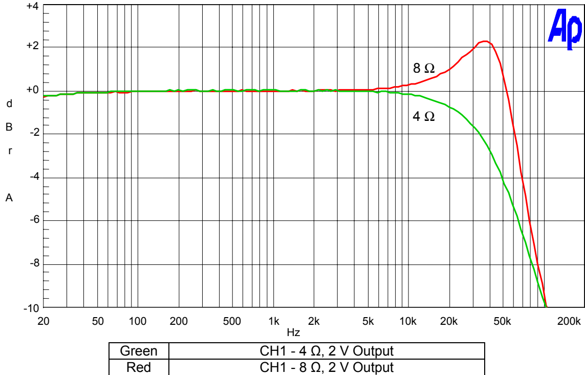
Figure 18. Frequency Characteristics vs. Load Impedance
