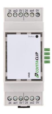
GSM-PRO I/O analogue output module, 4 analogue outputs 0 - 10V, Mounting type: Mounting rail TS 35, Supply voltage range: 20 V - 28 VDC
