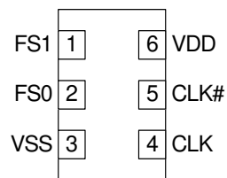
Figure 1. Pin Diagram - 6-pin Ceramic LCC
