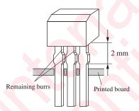
When soldering the leads, remember to separate the soldering position by 2 mm or more from the resin part of the package.
