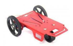
METAL ROBOT CHASSIS KIT WITH TWO WHEELS, TWO DC SERVO MOTORS, ONE FREE WHEEL.
