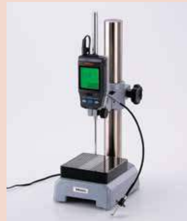
Application example using Digimatic Indicator ID-H.
