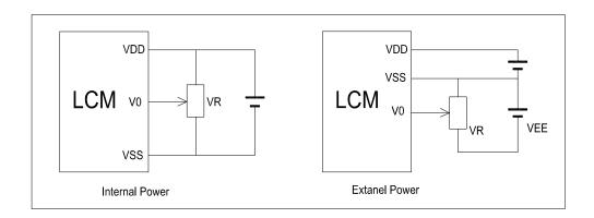
$V_{DD^{\sim}}V_0\text{: LCD Driving voltage}$
