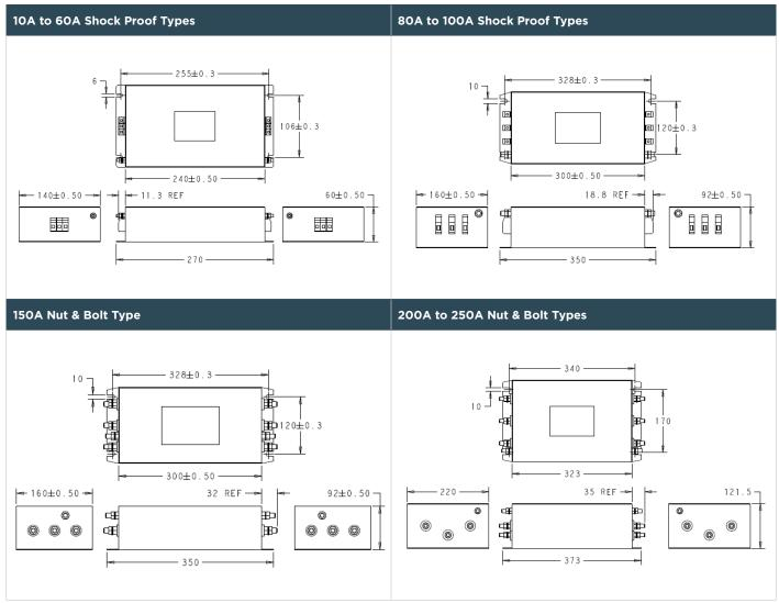
All dimensions in mm; Tolerances according: ISO2768-m
