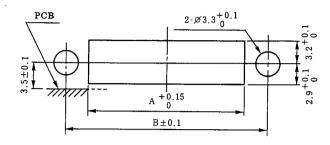
Unit: mm No. of HRS No. Part No. В Α CL231-3006-8 6 3110- 6S 18.06 23.96 CL231-3001-4 20.6 3110- 8S 26.5 CL231-3008-3 3110-12S 25.68 CL231-0018-0 3110-16S 30.76 36.66 CL231-0021-5 3110-14SB 28.22
