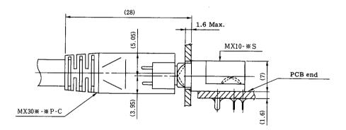
Note: Screw for Panel: M3 x 0.5 length 6 mm.
