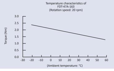
Temperature characteristics: Damper torque (rated torque in this document) varies according to the ambient temperature. As the temperature increases, the torque decreases, and as the temperature decreases, the torque increases. This is because the viscosity of the silicone oil inside the damper varies according to the temperature. The graph to the left illustrates the temperature characteristics.
