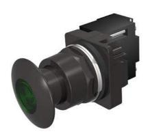
30mm BlackMax, Epoxy Coated Corrosion Resistant Complete Metal Unit Illuminated Push-Pull Operator Transformer type, 120V AC LED Lamp Mushroom Head Cap Small 1 3/4" (44.5 mm) Metal, Black with Green Lens 3 Position Momentary UL Listed, CSA Certified NEMA 1,3,3R,4,4X,12,13 & Automotive Standards
