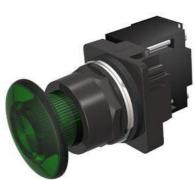
30mm BlackMax, Epoxy Coated Corrosion Resistant Complete Metal Unit Illuminated Push-Pull Operator Full Voltage, 6V AC/DC Incandescent Lamp Mushroom Head Cap Small 1 3/4" (44.5 mm) Plastic, Green 3 Position Pull-Momentary/Push-Maintained UL Listed, CSA Certified NEMA 1,3,3R,4,4X,12,13 & Automotive Standards
