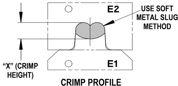
Use soft metal slug (solder) method to measure the "X" dimension. Verify tooling crimp height calibration by referring to the Go/No Go dimensions shown in the chart below.
