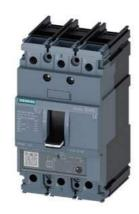
circuit breaker 3VA5 UL frame 125 breaking capacity class S 25kA @ 480 V 3-pole, line protection TM230, FTAM, In=20A overload protection Ir=20A fixed short-circuit protection Ii=7.5...15 x In UL489 SB (naval), 50 deg. cel. nut keeper kit on both sides
