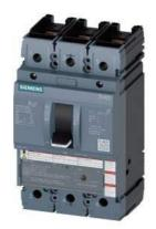
circuit breaker 3VA5 UL frame 250 breaking capacity class C 100kA @ 480 V 3-pole, line protection TM210, FTFM, In=200A overload protection Ir=200A fixed short-circuit protection li=10 x In nut keeper kit on both sides
