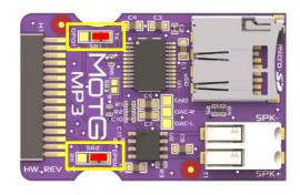
Unless the designer intends to use two UART MOTGS on a gen4-MOTG-AC2 or gen4-MOTG-AC4 board, the UART pins should be directed to TX, RX of the UMI as shown above.
