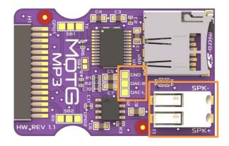
SPK+, SPK- provides a differential amplified output to a single speaker. Connect these pins to a 4/8/16/32-ohm speaker, at max of 3 watts when powered from a 5V supply. An 8-ohm 2.5W speaker is recommended.
