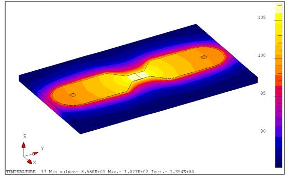
Track thickness 35  $\mu$ m, PCB thickness 1.6 mm,  $T_A = 85^{\circ}C$ , natural convection,  $I_{PN} = 10$  A rms or A DC.
