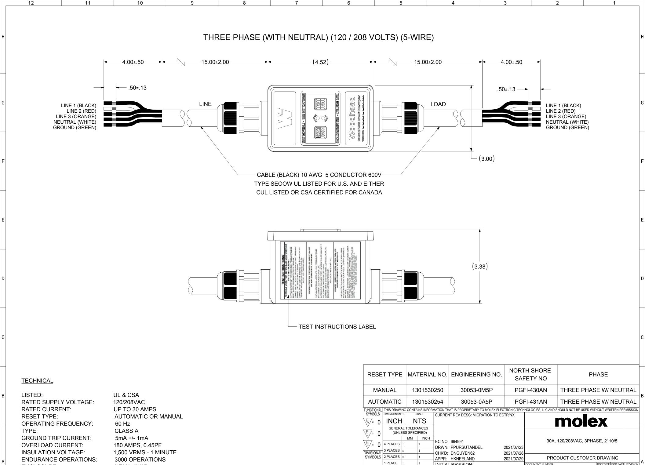
DRAFT WHERE APPLICABLE THIRD ANGLE PROJECTION DRAWING MUST REMAIN C-SIZE 130153 SEE TABLE DOCUMENT STATUS | P1 | RELEASE DATE | 2021/07/29 01:19:50 WITHIN DIMENSIONS 10
