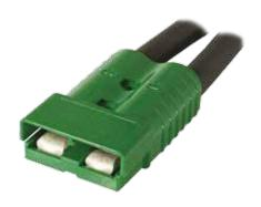
The SB\* 350 is the largest connector in the series with power capabilities up to 500 amps with a 350 mcm wire. Wires ranging from 1/0 to 350 mcm (53.5 to 185 mm²) fit into the one piece housing available in standard PC or a chemical resistant PBT/PC blend. Silver plated wire or busbar contacts minimize electrical resistance while offering supreme durability and reliability.
