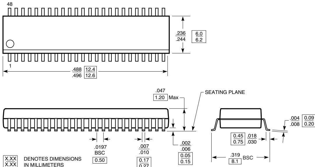
**Packaging Mechanical: 48-pin SSOP (V48)**
