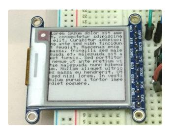
This time you will see the display going through a range of tests, from pixels, lines, text circles etc.
