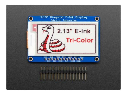
Easy e-paper finally comes to microcontrollers, with these breakouts, shields and friends that are designed to make it a breeze to add a tri-color elnk display. Chances are you've seen one of those new-fangled 'e-readers' like the Kindle or Nook. They have gigantic electronic paper 'static' displays - that means the image stays on the display even when power is completely disconnected. The image is also high contrast and very daylight readable. It really does look just like printed paper!
