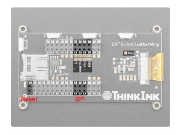
The FeatherWing uses SPI and some control pins for reading/writing data from the SD and then sending data to the E-lnk display
