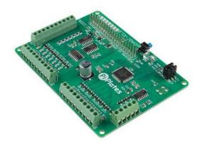
**Description:** The DAQCplate (Data Acquisition and Controller) from Pi-Plates adds a rich set of input/output options to your Raspberry Pi. It includes seven powerful digital outputs for driving external devices such as relays and high-current LEDs, as well as eight analog-to-digital inputs for measuring temperature, voltage, humidity and more. Additionally, there are eight digital inputs, two analog outputs and seven general-purpose indicator LEDs.
