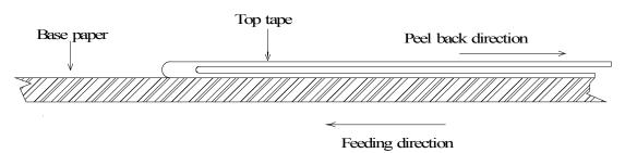
4.2 Base tape should not adhere to top tape when top tape is peeled back, and peel back direction is as follows.
