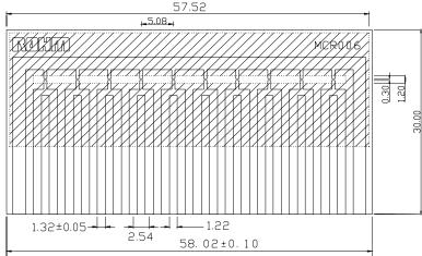
NOTE) \*1 The shaded area shows the solder resist treatment.
