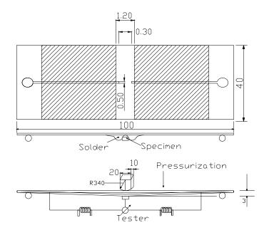
NOTE) \*1 The shaded area shows the solder resist treatment.
