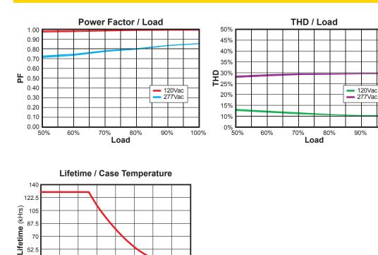
**Note:** The area under the life-temperature curve represents where the driver has highly reliable operation within specification. Driver performance may drift out of published specifications as the hours of operation exceed the curve at a given temperature. Higher operating temperatures increase the chances of a failure to function. Other electrical, mechanical and environmental factors affect driver lifetime but are not represented in this calculation.
