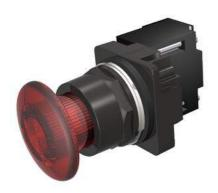
30mm BlackMax, Epoxy Coated Corrosion Resistant Complete Metal Unit Illuminated Push-Pull Operator Transformer type, 240V AC Incandescent Lamp Mushroom Head Cap Small 1 3/4" (44.5 mm) Plastic, Red 3 Position Pull-Momentary/Push-Maintained UL Listed, CSA Certified NEMA 1,3,3R,4,4X,12,13 & Automotive Standards
