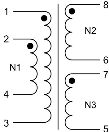
N1 denotes two windings connected in parallel. Terminals 1+2 and 3+4 must be tied as solder bridging is allowed.
