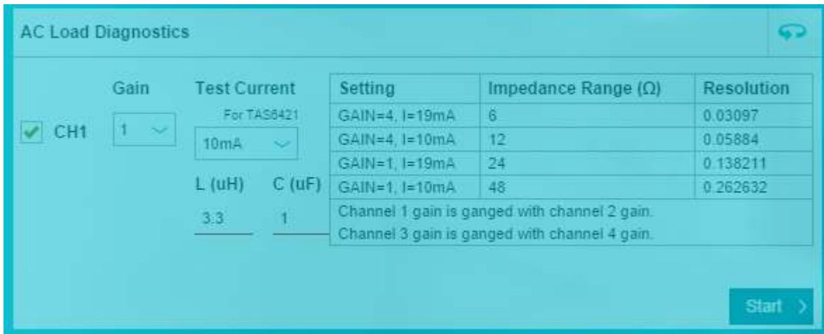
Figure 14. AC Load Diagnostics Section
