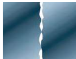
Typical interference fit has 30% metal-to-metal contact.
