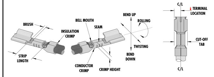
Terminal is to be centrally located between the two (2) cut-off tab edges by one half of the total cut-off tab tolerance. This illustration is a generic terminal representation and not an exact image of any terminal listed in the scope.
