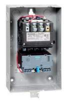
Non-reversing motor starter, Size 1, Three phase full voltage, Solid-state overload relay, OLR amp range 0.25-1A, Non-combination type, Enclosure type 1, Indoor general purpose use, Standard width enclosure
