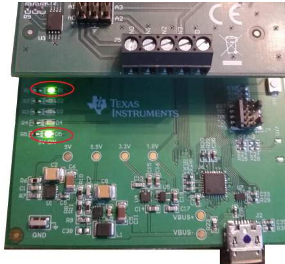
Figure 3-4. LED Indicators D1 and D5
