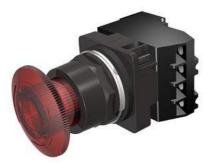
30mm BlackMax, Epoxy Coated Corrosion Resistant Complete Metal Unit Illuminated Twist-to-Release Transformer type, 120V AC Incandescent Lamp Mushroom Head Cap Small 1.79" (45 mm) Plastic Cap, Red 2 Position Maintained, Twist-to-Release with 1 N.O. - 1 N.C. Heavy Duty Contacts, A600/P600 UL Listed, CSA Certified NEMA 1,3,3R,4,4X,12,13 & Automotive Standards
