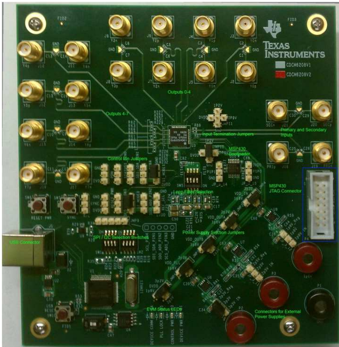
Figure 1. CDCM6208 Evaluation Board
