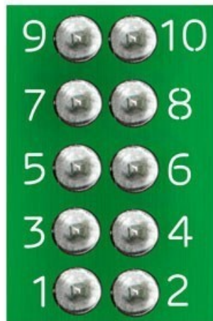
Figure 3.3b Connection of the Intersil ZLUSBREF02 PMBus-to-USB adapter (connector is found on the back side of the ROA 128 3835 board)
