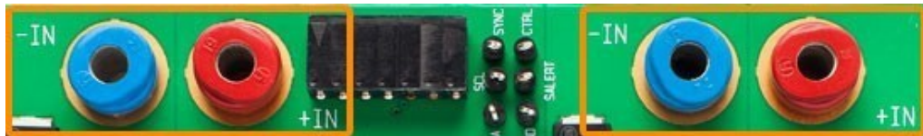
Figure 3.1 Connect 48V between the “-IN” and “+IN” DC power connectors located on the same side of the board (see orangerecangles)
