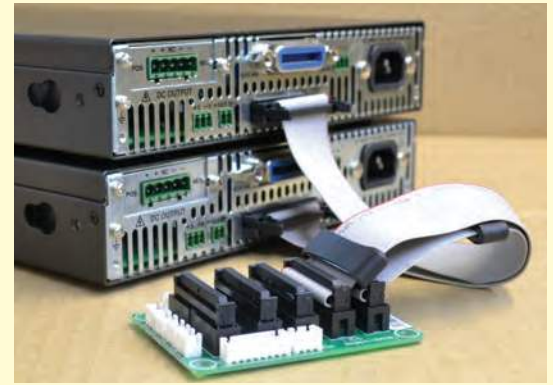
Parallel connection of two identical KLN power supplies (up to five possible) using optional Parallel Socket Board 536-0129 and Programming Port Cable 518-0119
