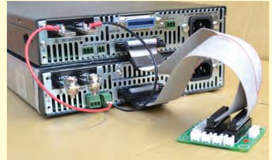
Series connection of two identical KLN power supplies using optional Series Socket Board 536-0130 and Programming Port Cable 518-0119
