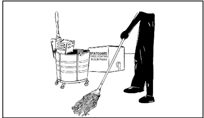
Figure 7. Applying floor finish
