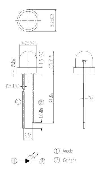
Note: Tolerances unless dimensions ±0.25mm
