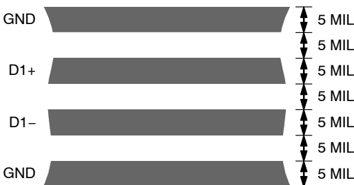
Figure 17. Arrangement of Signal Tracks
