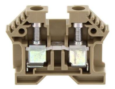
Feed-through terminal for direct mount/block variant, Screw connection, Mounting type: Mounting surface, Rated cross-section: 10 mm<sup>2</sup>, Width: 8 mm, Colour: Beige
