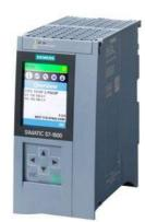
SIMATIC S7-1500F, CPU 1516F-3 PN/DP, central processing unit with 1.5 MB work memory for program and 5 MB for data, 1st interface: PROFINET IRT with 2-port switch, 2nd interface: PROFINET RT, 3rd interface: PROFIBUS, 10 ns bit performance, SIMATIC Memory Card required
