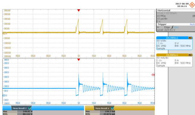
Figure 29 – 85 VAC Input. Condition: 3.8 V – 20 mA, 12 V – 0 A. Upper: I_{DRAIN} , 50 mA / div. Lower: V_{DRAIN} , 50 V / div., 10 \mu s / div.
