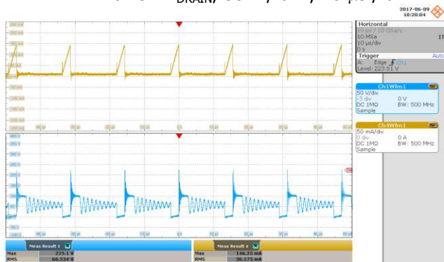
Figure 31 – 85 VAC Input. Condition: 3.8 V – 20 mA, 12 V – 20 mA. Upper: I_{DRAIN} , 50 mA / div. Lower: V_{DRAIN} , 50 V / div., 10 \mu s / div.
