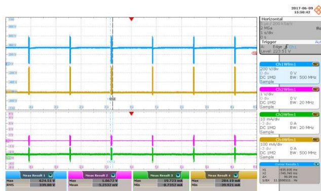
Figure 44 – 265 VAC Input. Condition: 3.8 V – Shorted, 12 V – 0 mA. Auto-Restart: 91 ms. Upper: V_{DS} , 200 V / div., 1 s / div. Upper Middle: I_{DS} , 100 mA / div. Lower Middle: V_{OUT3.8} , 1 V / div. Lower: I_{OUT3.8} , 10 mA / div.
