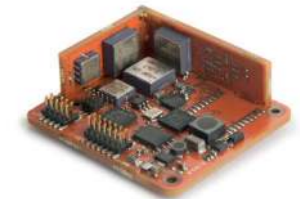
MTi OEM: 37x33x12 mm, 11g, 16-pins header
