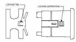
LOCKING TAB MUST ALIGN WITH LOCKING SERRATIONS
