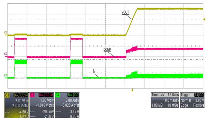
Figure 10: Hiccup Mode and Recovery (to 5.0 V at 0.5 A, for A8585/A8585-2, shown)
