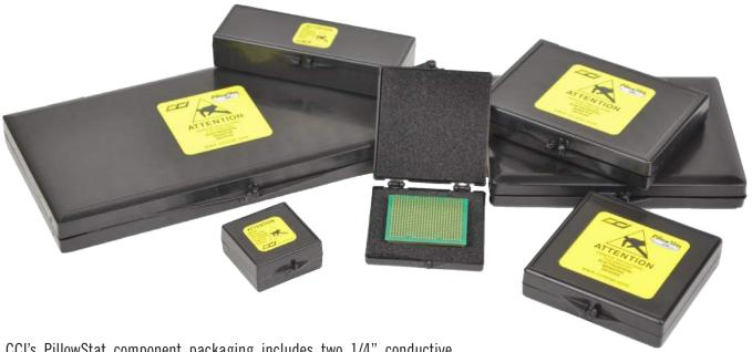
CCI's PillowStat component packaging includes two 1/4" conductive foam "pillow pads" (PP2020 has two 1/8" pillow pads & PP1030 has an additional 1/8" pillow pad) inside a static shielding solid plastic box. This package is designed to safely package one or more ESD sensitive devices without custom tooling. Ball grid arrays, wafers, and components with fine pitched leads are possible applications.
