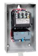
Non-reversing motor starter Size 1 Three phase full voltage Solid-state overload relay OLRelay amp range 0.75-3.4A 240VAC 50HZ / 277VAC 60HZ coil Combination type Indoor general purpose use
