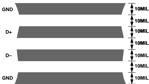
Figure 18. Arrangement of Signal Tracks
