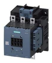
power contactor, AC-3 185 A, 90 kW / 400 V AC (50-60 Hz) / DC operation 110-127 V AC/DC auxiliary contacts 2 NO + 2 NC 3-pole, frame size S6 busbar connections drive: conventional spring-loaded terminal
