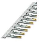
Crimp contact, Socket, rolled, Taped articles, number of pieces per reel: 500, contact diameter: 1 mm, crimp range:  $0.22 \text{ mm}^2 \dots 0.56 \text{ mm}^2$ , Item is lead-free in accordance with RoHS II without Exemption 6c (Pb <0.1%)
