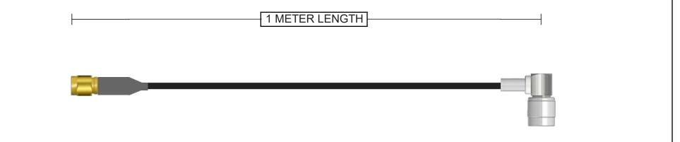
Connector A 132113RP SMA Plug Straight Brass Gold + Heatshrink 50 Ohm RG-58 Continuity/Hi-Pot Connector B 122140 TNC Plug Right Angle Brass Nickel
